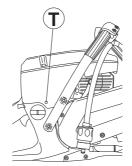
Rec. idle speed: 2700 rpm
